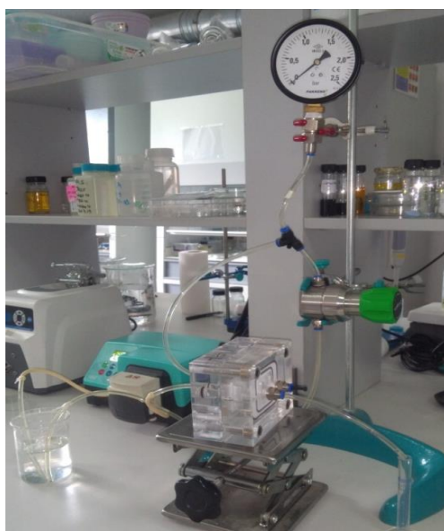
Figure 2.4. MWCO test in crossflow module
